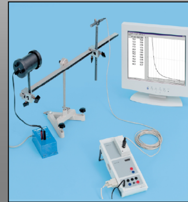
Determining the luminous intensity as a function of the distance from the light source – Recording and evaluating with CASSY
