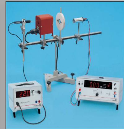
Stefan-Boltzmann law: measuring the radiant intensity of a "black body" as a function of temperature
